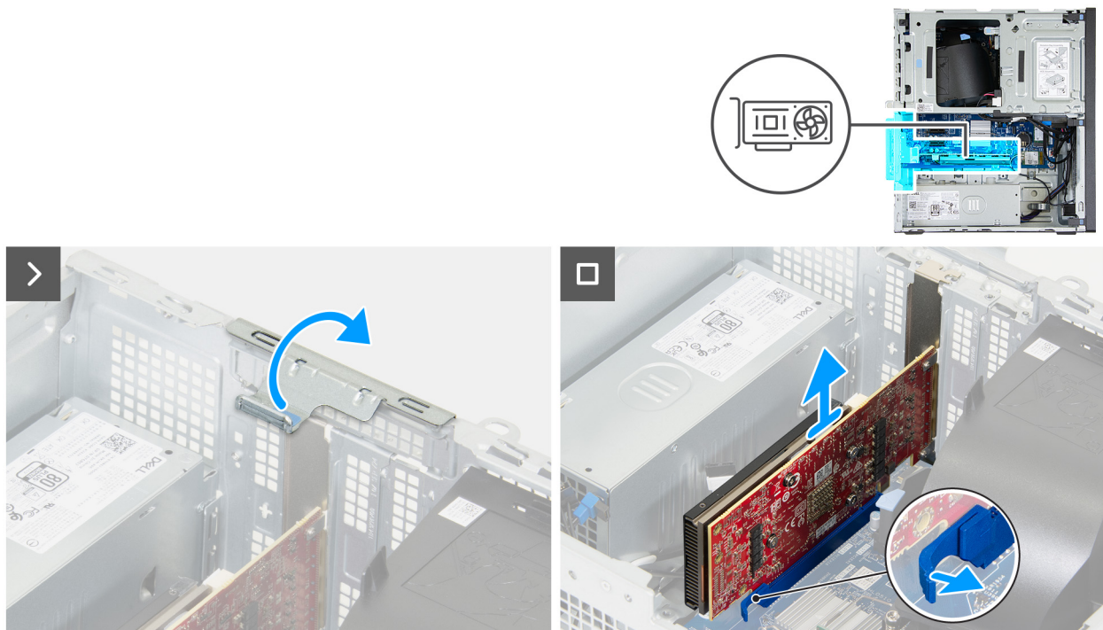
Figure 34. Removing the graphics card
