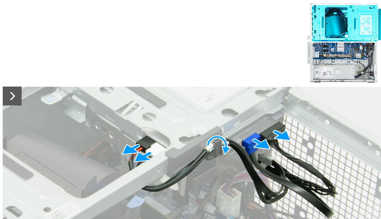
Figure 42. Removing the drive bay
