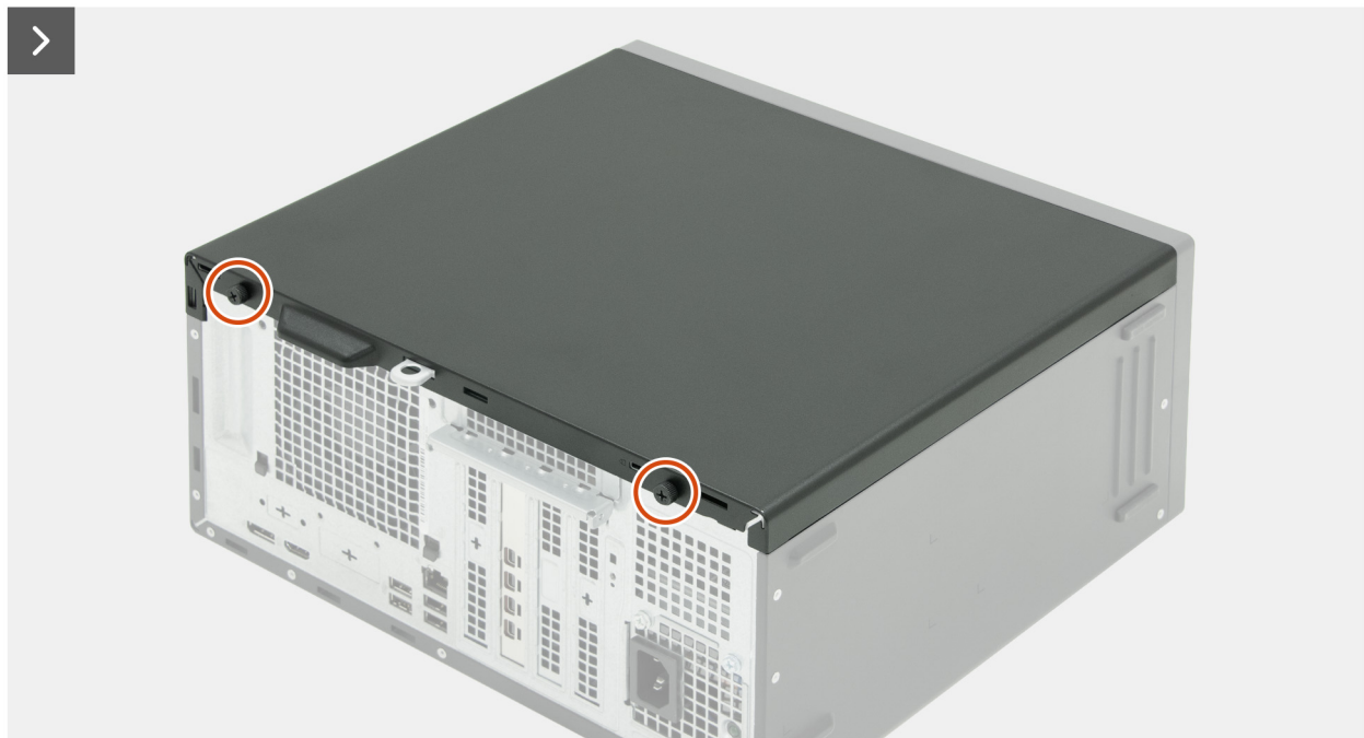
Figure 13. Removing the left-side cover
