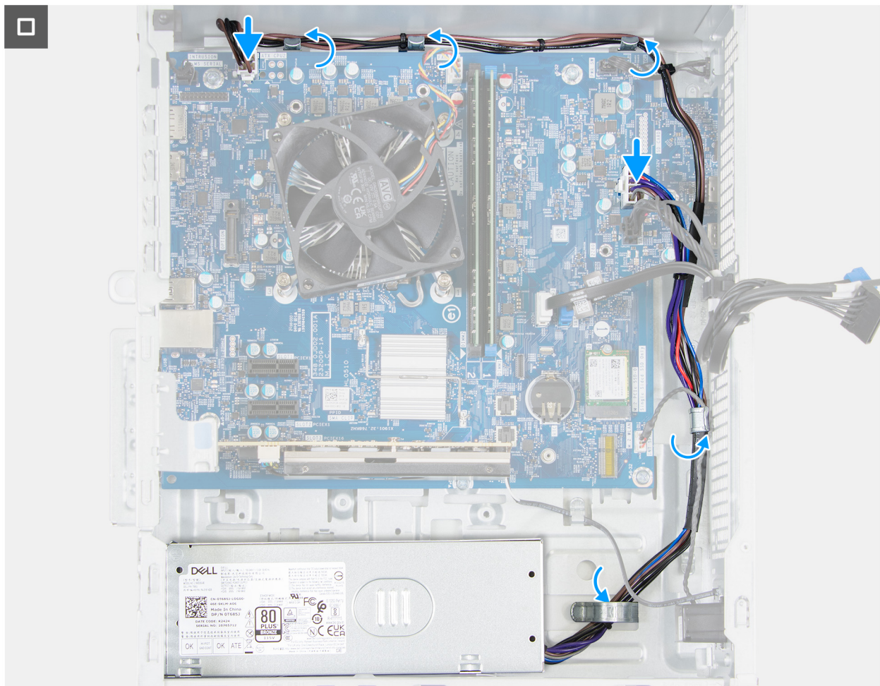
Figure 65. Installing the power-supply unit
