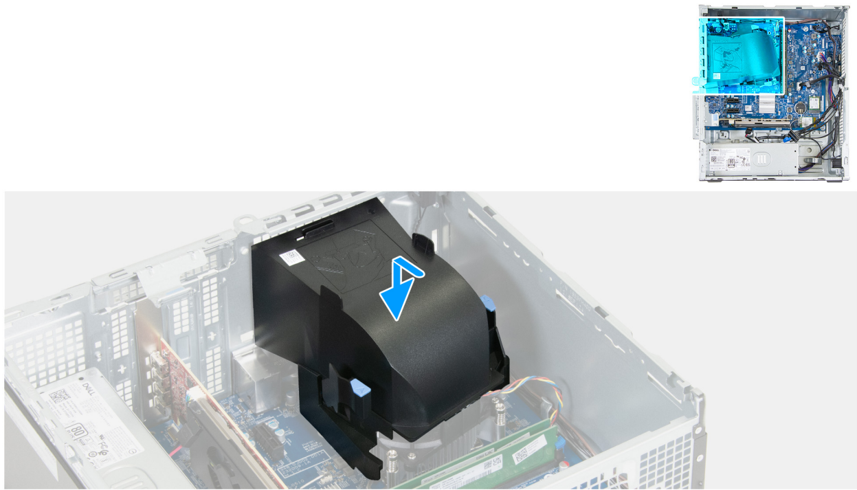
Figure 53. Image: Installing the fan shroud
