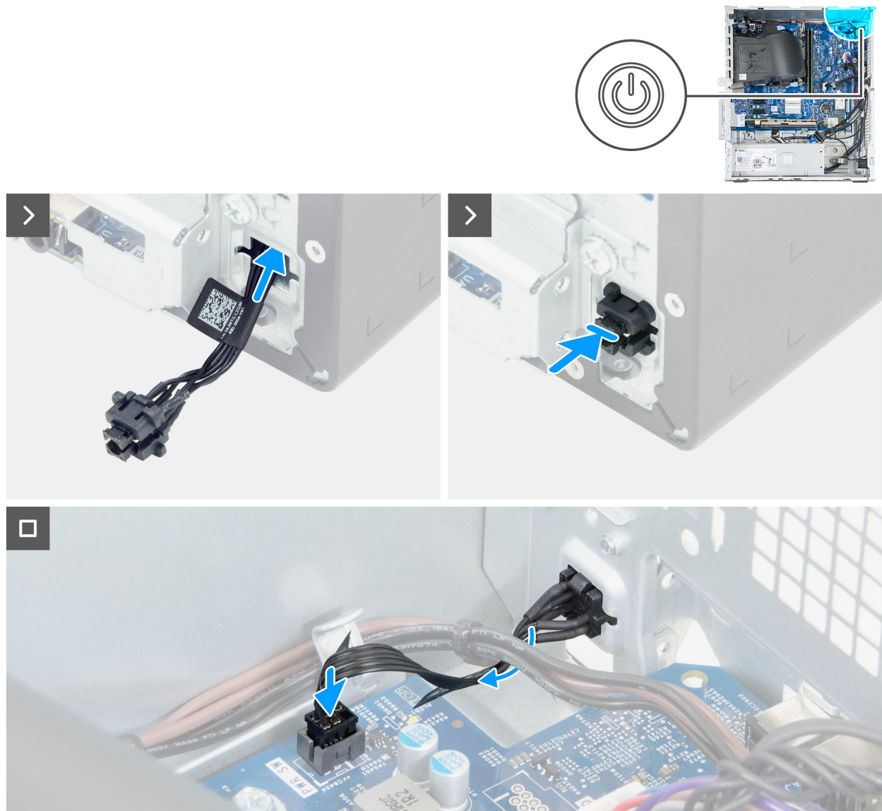
Figure 51. Installing the power button
