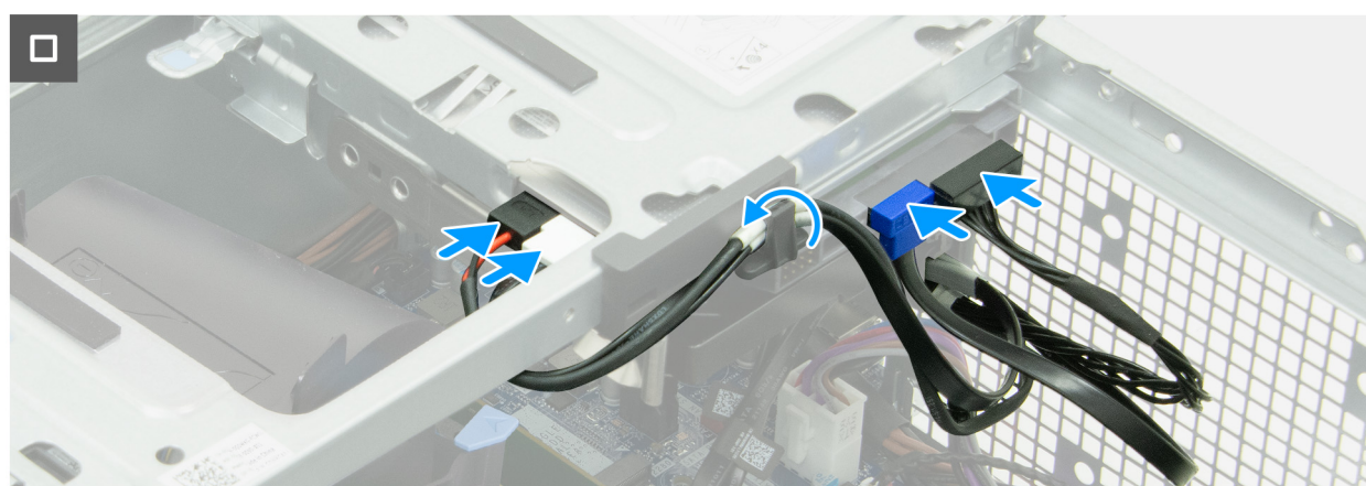
Figure 45. Installing the drive bay
