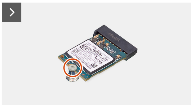
Figure 29. Removing the M.2 2230 solid-state drive
