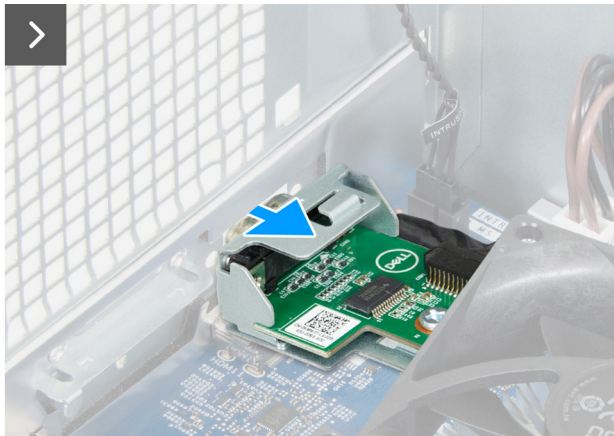
Figure 57. Removing the serial-port module
