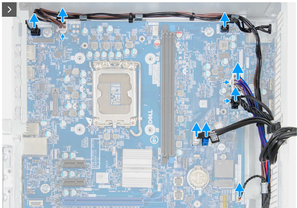
Figure 72. Removing the system board
