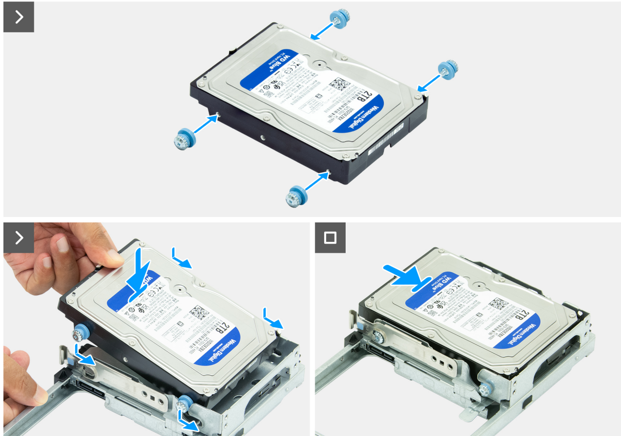
Figure 40. Installing the hard drive
