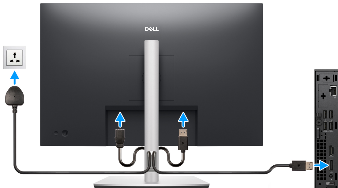
Figure 6. Connect the display
